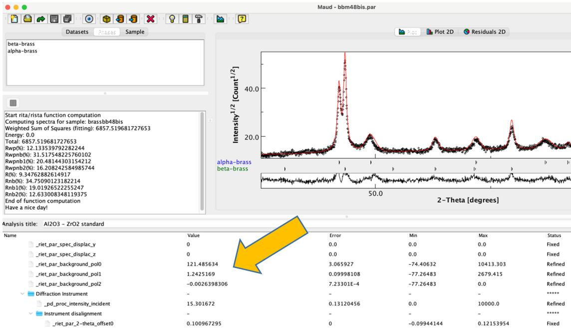
b- Adjust manually amap the 3 Background parameters to superpose measured and calculated XRD spectra
